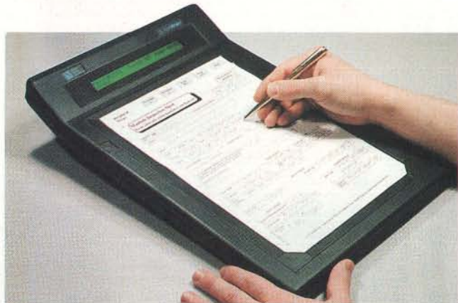
The ScriptWriter II electronic clipboard lets you create a computer record and an original paper copy simultaneously.
